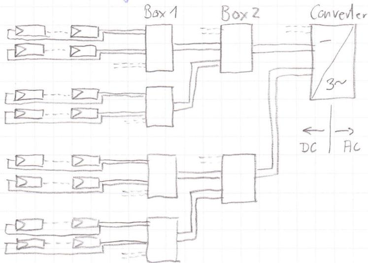
Voltage Drop :  $\Delta U = 2 \cdot I \cdot R$  ;  $R = \frac{l}{30 \cdot A}$  ;  $\kappa_{Cu} = \frac{56 \text{ m}}{\Omega \cdot \text{mm}^2}$
